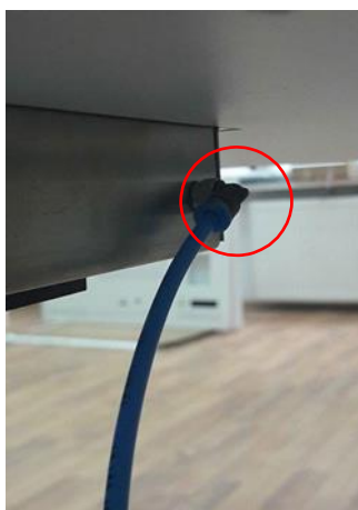
Figure 34.9 Gas line connection under the tabletop
