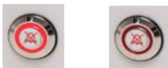
Figure 13.1 Alarm key which indicates the alarm condition
