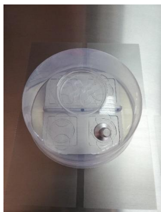
Figure 11.8 Gas hood placed over the gas nozzle
